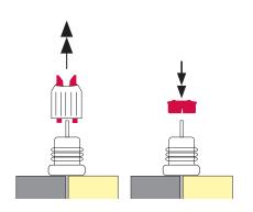
Shake unit well (1 minute +) Allow unit to sit upright for several minutes to de-air. Unscrew lock nut and remove plug. Insert Flow Restrictor into Top Ports.
