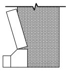
PLACE END OUTLET OVER BOTTOM CORNER OF COMBINATION DRAIN WITH FABRIC UP
