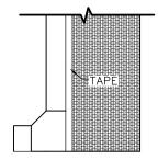
FOLD FABRIC AROUND EXPOSED EDGE OF CORE AND TAPE WITH 3" UNDERGROUND RATED TAPE
