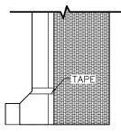
SECURE ALL EDGES WITH 3" UNDERGROUND RATED TAPE TO PREVENT SOIL INTRUSION
