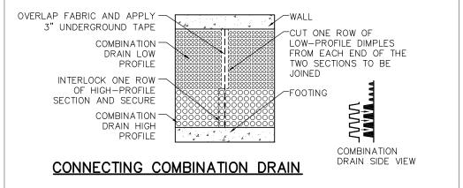
INSTALL THE FIRST ROW OF COMBINATION DRAIN AT THE BASE OF THE WALL WITH THE HIGH-PROFILE SECTION ATOP THE FOOTING.
