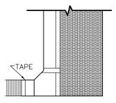
INSERT 4" PIPE INTO END OUTLET AND SECURE CONNECTION WITH 3" UNDERGROUND RATED TAPE
