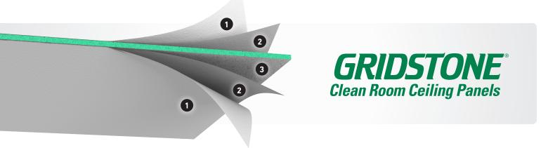
Gridstone Clean Room Gypsum Ceiling Panels feature a vinyl laminate on the top and bottom and sealed edges to help maintain low levels of airborne particulates in clean rooms, server rooms and other areas requiring high levels of cleanliness.
