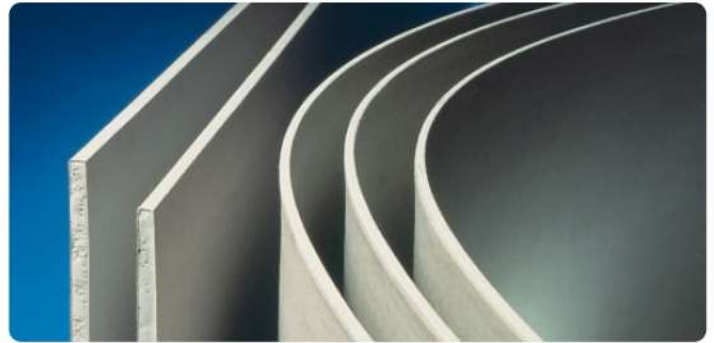
High Flex Gypsum Board is significantly more flexible in the vertical direction (long edges parallel to the framing) than in the horizontal direction (see table).
