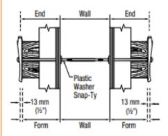
Plastic Washer break back is 3 mm to 5 mm (1/8" to 3/16") less than the plastic washer thickness.
