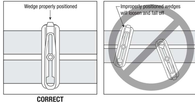
The Ty Head must not be positioned lower than the midpoint of the wedge. The proper Ty Head position is at the midpoint of the wedge slot, or higher.
