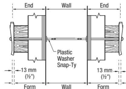
Plastic Washer break back is 3 mm to 5 mm (1/8" to 3/16") less than the plastic washer thickness.
