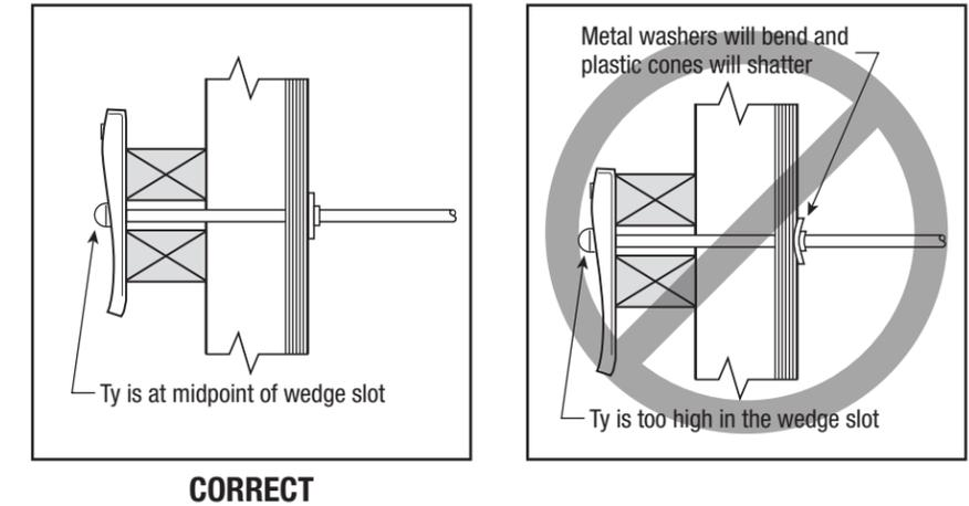
To achieve proper form structures, it is important that all form tys are installed and used properly. Excessive loads will be transferred to adjacent tys and can result in form failure if tys and/or their required hardware are omitted. Ensure that form tys are properly aligned. Increased loads placed on form tys because of misalignment may cause form failure to occur. Also, reduced load capacities can result from form tys damaged because of misalignment during installation.
