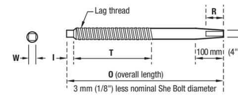
Variable 2400 mm (8'-0") to 3000 mm (10'-0") Lift Form using She Bolts with High Tensile Lagstud
