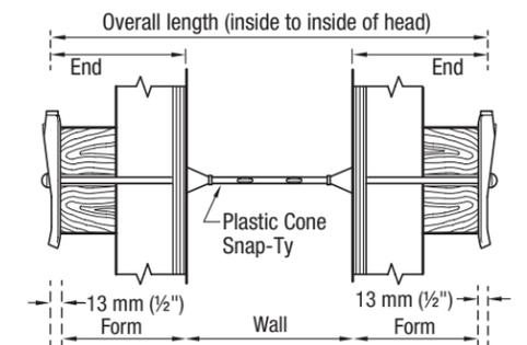
For architectural design, insert the Plastic Snap-Ty Plug once form work has been removed.
