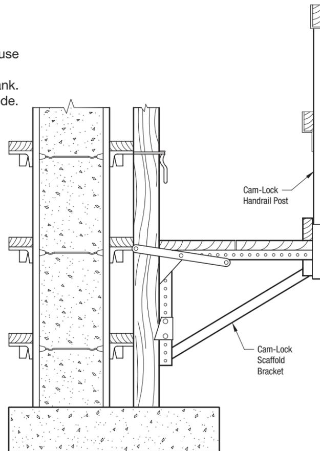
Not to be used above 6.0 m (20'-0"). Any scaffolding above six metres (twenty feet) should be checked with local, provincial code requirements.
