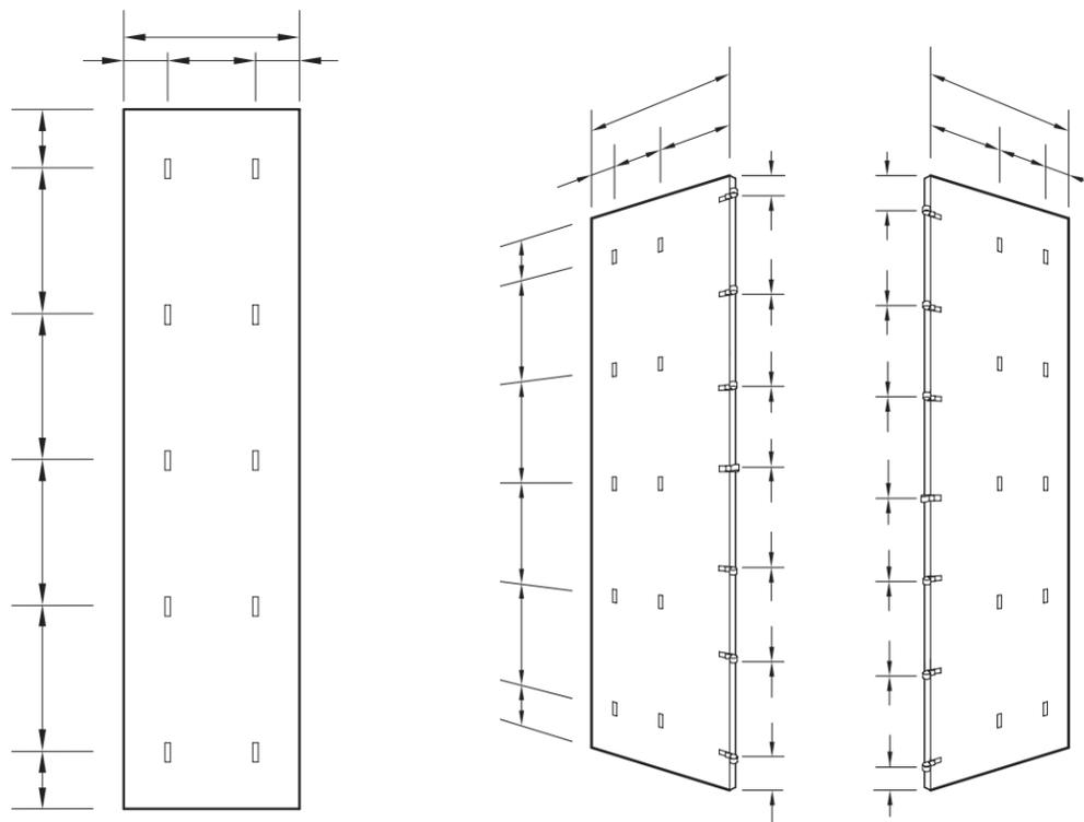
Corners are made from  $\frac{3}{4}$ " plywood, and hinges supplied by AR. Corner shown is the standard 2' and works best on most jobs. Corners are connected by inserting a  $\frac{5}{8}$ " rod through the hinges.
