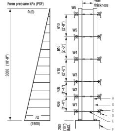
Typical 6100 mm (20'-0") High Wall Formwork,
