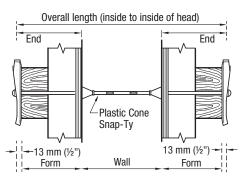
For architectural design, insert the Plastic Snap-Ty Plug once form work has been removed.
