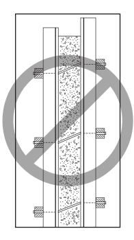
Wales may be crushed or washers may bend if too much space is allowed between the walers. Too much space causes the form to move outward and will result in incorrect wall thickness and spreader cones becoming trapped in the concrete. Incorrect wall thickness can also be caused from washers being deflected due to the increased lateral form pressure.
