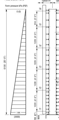
**LEGEND** A = 19mm (%") plywood **B** = 38X89 (2X4) studs @ 200 (8") on centre **C** = Two 38X89 (2x4) walers **D** = Tywedge (sweg-H) **E** = Snap-ty or Space-TyTM **F** = Footing **G** = 38X89 (2x4) studs @ 150 (6") on centre **H** = 38X89 (2x4) studs @ 100 (4") on centre
