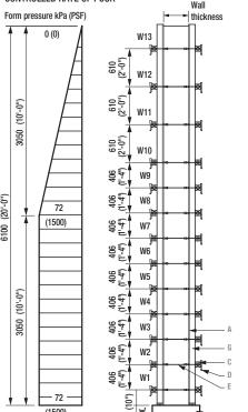
Snap-Ty 10 kN (2,250 lbs) spacing: W1 to W10 @ 305 (12") on centre W11 @ 406 (1'-4") on centre W12 and W13
