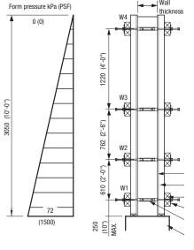
Typical 6100 mm (20'-0") High Wall Formwork, FULL LIQUID HEAD
