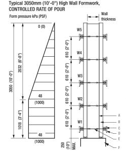
Snap-Ty 10 kN (2,250 lbs) spacing: W1, W2 and W3 @ 305 (12") on centre
