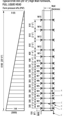
Snap-Ty 10 kN (2,250 lbs) spacing: W1, W2 and W3 @ 305 (12")
