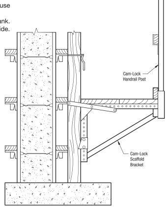
Not to be used above 6.0 m (20'-0"). Any scaffolding above six metres (twenty feet) should be checked with local, provincial code requirements.
