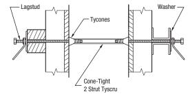
The minimum Lagstud Bolt length required is equal to the sum of the flat washer, waler studs, form ply, set back and the coil length plus 13 mm ( $\frac{1}{2}$ ").
