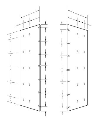
Corners are made from ¾" plywood, and hinges supplied by AR. Corner shown is the standard 2' and works best on most jobs. Corners are connected by inserting a 5/8" rod through the hinges.
