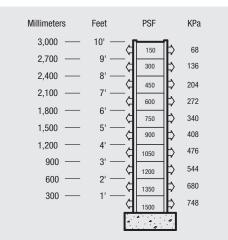
As you increase the height of plastic concrete to the forms, the pressure will build at a rate of 150 PSF per foot of depth. This will be true as long as all concrete remains in a plastic state.
