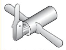
Caution: Do not use the Tightening Wrench for straightening forms or for pulling smooth rods from set concrete.
