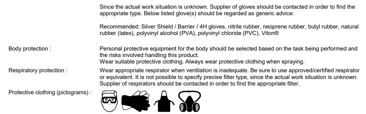
Note: Application of paint products by spraying requires additional safety precautions: Full body suit, Full face respirator with air supplied.
