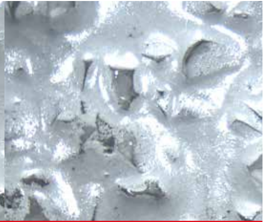
Auto-Gard T Controlled abrasion test: aggregate bonds to coating.
