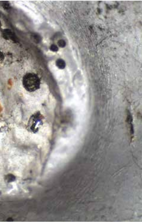
Traditional Aggregate Controlled abrasion test: notice "Pop Out" of aggregate
