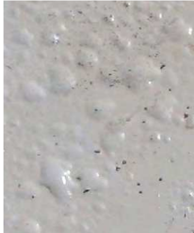
Blisters due to trapped solvent
