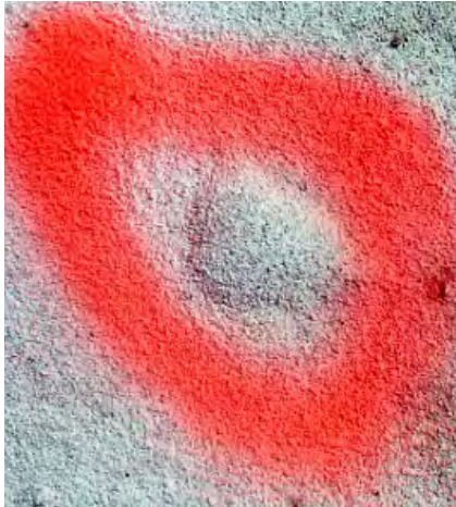
Blister due to contamination
