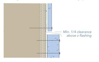
Block out penetrations with flashing over the top edge of the block. Keep a ¼" clearance between the siding and flashing.
