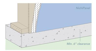
All horizontal trim is required to be flashed with a ¼" clearance between the siding and z flashing. Do not caulk the clearance gap.
