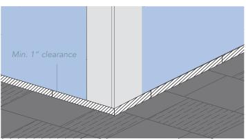
A kickout flashing must be present at roof to wall intersects in order to direct roof water away from the siding and trim. Include drip edge flashings to protect fascias/trim below roof edges.
