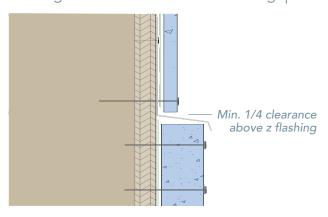
At roof and wall junctures and according to roofing manufacturer's instructions, flashing and counter-flashing are required. Panels must be installed with a minimum 1" clearance from roofing.
