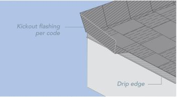
Block out penetrations with flashing over the top edge of the block. Keep a ¼" clearance between the siding and flashing.
