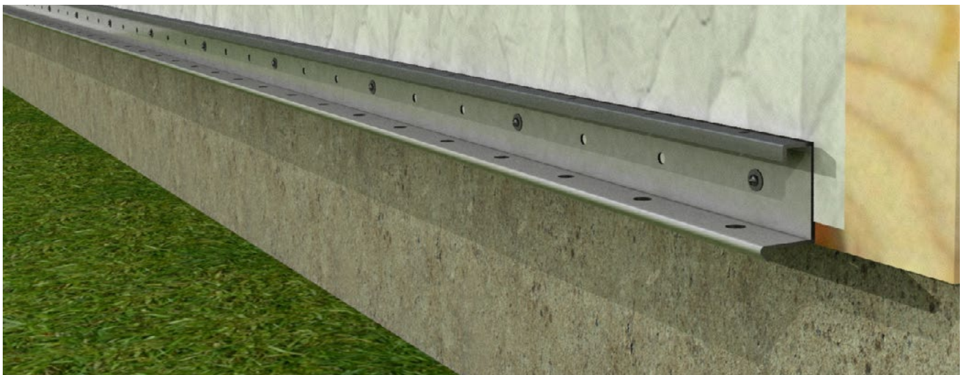
Vertical (Panel) Starter Track fastened every 6" to 9" (152-229mm) to framing.
