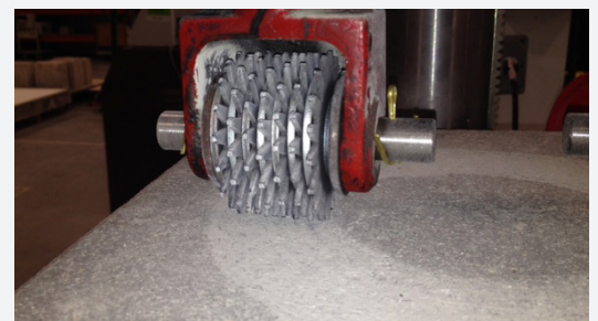
The ASTM C779 Procedure B uses steel dressing wheels to test the abrasion resistance of concrete surfaces. (Source: Nelson Testing Laboratories)
