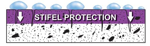
Winter is rough on concrete and rougher still in regions where frequent freeze/thaw cycles are common. If water penetrates the concrete's surface and then changes to ice, the results can be surface scaling. Additionally, corrosive road salts combined with the freeze/thaw cycles can cause untreated surfaces to suffer surface delamination, spalling and scaling.
