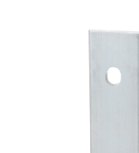
Flat Bar 1" (25mm) wide, .090" (2.3mm) thick. Punched 6", 8", or 12" (150, 200 or 300mm) o.c. Terminates single-ply membrane at parapet walls.
