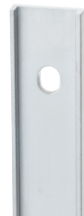
Channel Bar 1" (25mm) wide, .100" (2.5mm) thick. Punched 6", 8", or 12" (150, 200 or 300mm) o.c. Terminates single-ply membrane at parapet walls.
