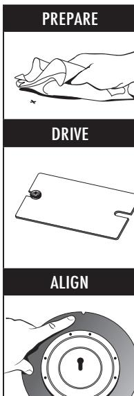
**1.** Mark location where PowerGrip Plus is to be installed. Prepare membrane surface at each location following roof system manufacturers' requirements.
