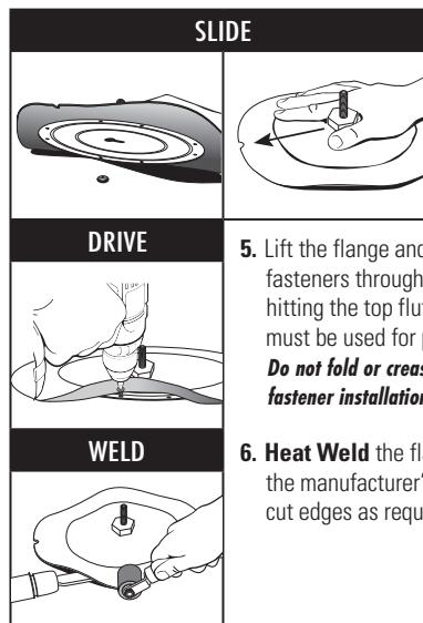
**4.** Slide the PowerGrip Plus into place over the head of the fastener.
