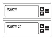
**OPTION: SET ALARM** activates an alarm that signals the end of a completed weld. Press Select to activate the option. Press ▲ or ▼ to choose Alarm On or Alarm Off mode. Press Select to accept the mode and exit.
