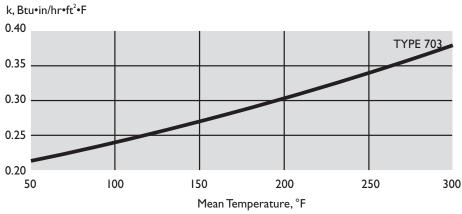
Apparent thermal conductivity curve determined in accordance with ASTM Practice C1045 with data obtained by ASTM Test Method CI77. Values are nominal, subject to normal testing and manufacturing tolerances.
