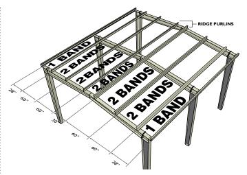
2. Position each band off of the purlins equal to ¼ of the purlin spacing for all spacings greater than 30 inches. For spacings less than 30 inches, divide the cavity in half.
