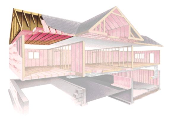
Before you add any insulation to your attic, you need to know how much insulation (R-value) is already there. This is simply done by measuring the thickness of your attic's existing insulation. Most older homes have between 3" and 6" of fiber glass blanket insulation. This is roughly equal to an R-value between R-9 and R-19.
