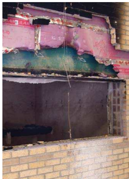
FOAMULAR® XPS with brick veneer stripped away above the test window showing limited damage and minimal fire spread after the NFPA 285 fire test.
