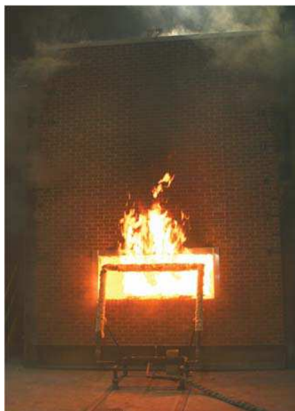
Fire emitting from the NFPA 285 test window.
