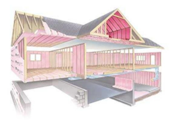
The rafters in cathedral ceilings are usually made of 2x12s or 2x10s, and Owens Corning makes two special high-density insulation products specifically for these rafters -- R-38C for 2x12s and R-30C for 2x10s. These products are appropriate for cathedral ceilings because the R-38C batt is 10 1/4 inches thick, which leaves over one inch of vent space for free air flow in a 2x12 joist. The R-30C batt, at 8 1/4 inches thickness, is designed to do the same thing in a 2x10 joist.
