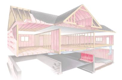
In a heated crawlspace or one with uninsulated ducts or water pipes, the walls should be insulated. R–19 PINK fiber glass insulation or R–25 MIRAFLEX® insulation work best for this. MIRAFLEX R–25 insulation's poly wrapping and compact roll size make it easy to handle and install, especially in a confined area like a crawlspace.
