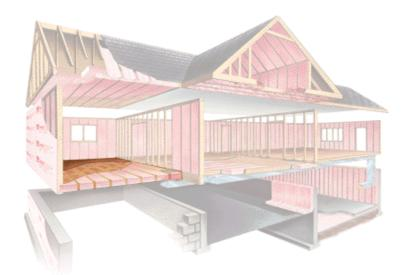
A lot of energy can leak through the floor, so it's important to insulate it correctly. R-19 or R-25 fiber glass batts can be installed in floor applications.
