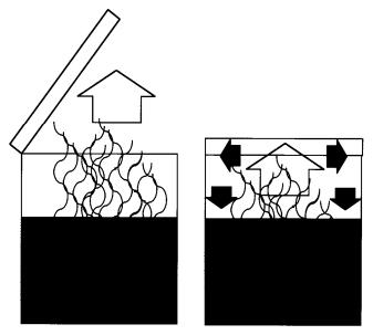
When kettles were left open (left), light oils boiled off and escaped to the atmosphere, thereby raising the softening point of the asphalt. With kettles closed (right), as is now required by environmental regulations, the boiledoff oils condense on the inside of the kettle and "fallback" into the asphalt-which decreases its softening point.
