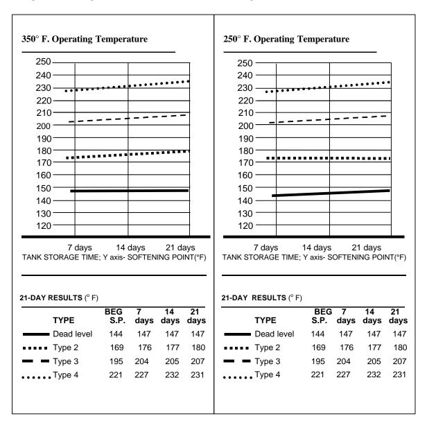
NOTE: The reasons that softening points tend to increase during long-term, lower-temperature storage are: (1) storage tanks must be vented, and in that condition, light oils can
