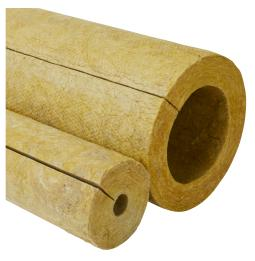
Owens Corning<sup>®</sup> Thermafiber<sup>®</sup> Pro Section WR, made with Paroc<sup>®</sup> technology, is a water repellent mineral wool pipe insulation engineered to meet the toughest industrial specifications and conditions. It is capable of withstanding high temperatures, conserving energy, and reducing noise. Thermafiber<sup>®</sup> Pro Section WR is designed for use on high temperatures pipework in process industries and fire resistant applications.
