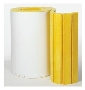
Fiberglas<sup>™</sup> Pipe and Tank Insulation is made of semi-rigid fibrous glass board material, factory-jacketed with an FRK or ASJ Max jacket. The insulation is adhered with the end grain perpendicular to the jacket. This provides a flexible product that is easily wrapped around pipes, tanks or irregularly shaped objects, while providing good rigidity and abuse resistance.
