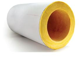
Owens Corning<sup>®</sup> Large Diameter Fiberglas<sup>™</sup> Pipe Insulation is molded of heavy density resin bonded inorganic glass fibers that come in one-piece, 36" (914mm) long, hinged sections. Sections begin at 18" O.D. through 42" O.D. and can be ordered as factory applied SSL<sup>®</sup> with ASJ Max or as unjacketed No-Wrap.
