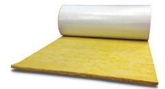
Fiberglas<sup>™</sup> FLEXWRAP<sup>®</sup> is a flexible insulation product made from fiberglass blanket bonded together with a thermosetting resin. The fibers are oriented to provide good compressive strength while providing flexibility during installation. FLEXWRAP<sup>®</sup> insulation is suitable for operating temperatures up to 850°F (454°C). Available in ASJ or FRK facings.
