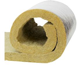
Thermafiber<sup>®</sup> Industrial Wrap, made with Paroc<sup>®</sup> technology, is a mineral wool wrap capable of withstanding high temperatures and is designed to be used in industrial equipment and applications. This product is used to insulate large diameter piping, vessels and ducts. Thermafiber<sup>®</sup> Industrial Wrap is available with or without a reinforced alulaminate facing.
