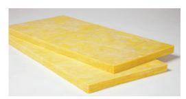
Fiberglas<sup>™</sup> SCR Insulation Board is a lightweight insulation board composed of resilient, inorganic glass fibers bonded with a thermosetting resin. SCR Board is designed specifically for use on selective catalytic reduction units (SCR) in powerplants.
