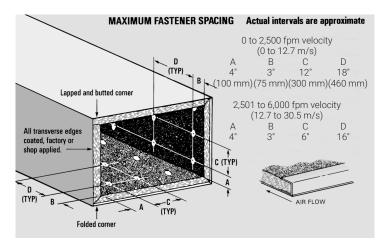
**Figure 1:** Metal nosing (channel or zee) must be used where liner is preceded by unlined metal. Otherwise, when air velocity exceeds 4,000 fpm (30.5 m/s), use metal nosing on all upstream edges of duct liner.
