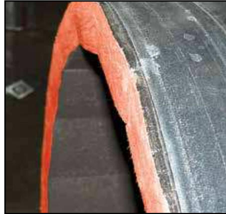
Figure 14 - \frac{1}{8} " additional liner on couplings and fittings
