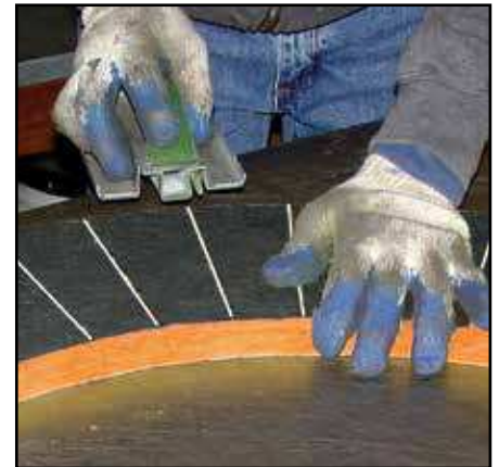
Figure 27 - Hand grooving reducer lines
