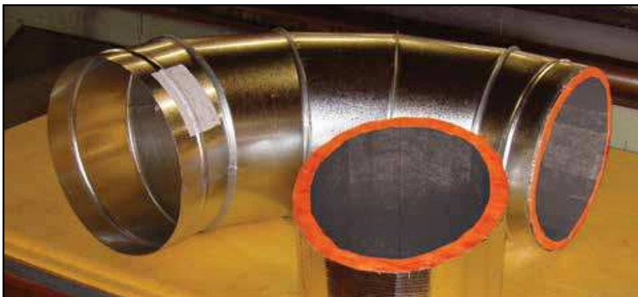
Figure 17 - Prepared end gore for elbow
