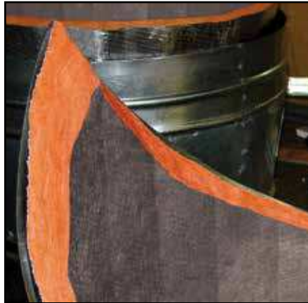
Figure 19 - Trimmed branch leg of Tee
