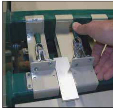
Figure 2 – Spacing with a gage block
