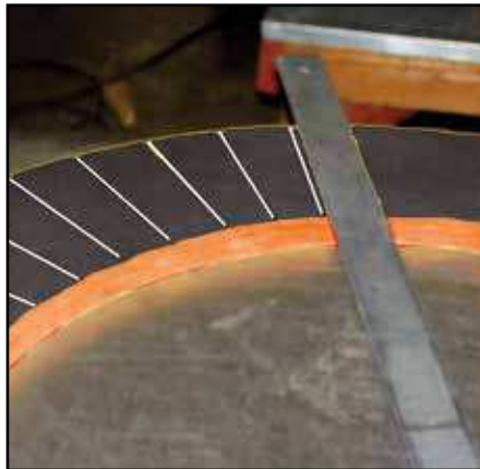
Figure 26 - Marking out groove lines
