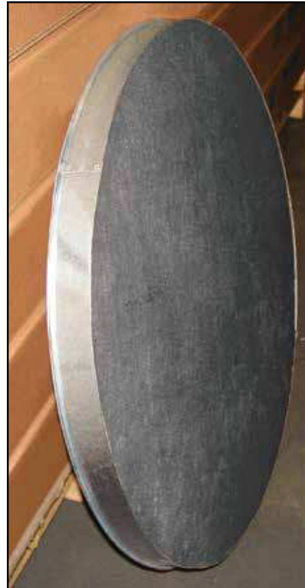
Figure 31 - View of insulated end cap
