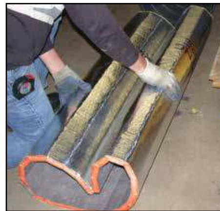
Figure 10 - Heart shape for insertion into duct
