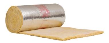
SOFTR\* Duct Wrap is a blanket of glass fiber insulation factory-laminated to FRK vapor retarder facing. A 2" (50mm) stapling and taping flange is provided on one edge. This product is designed to meet existing performance standards such as NFPA 90A and 90B and other mechanical and energy codes. SOFTR\* Duct Wrap FRK flexible design makes it easy and fast to install, helps prevent duct condensation, and increases building occupants thermal comfort.
