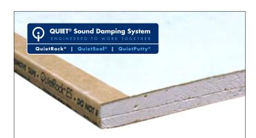
Mold resistant, Type X , 5/8" sound damping gypsum panel without paper or metal in the core. Cuts and installs similar to standard gypsum panel products. QuietRock® ES Mold Resistant is recommended for mold sensitive applications such as schools, hospitals, and government projects.
