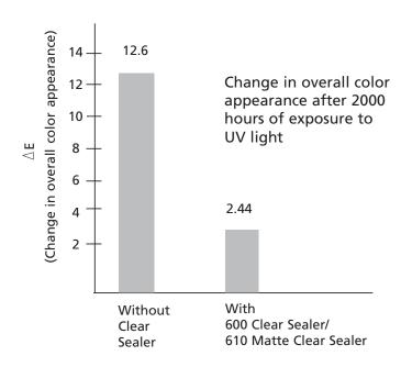
Finishes coated with 600 Clear Sealer/610 Matte Clear Sealer show far less change in overall color than finishes without 600 Clear Sealer/610 Matte Clear Sealer after 2000 hours of intense laboratory UV exposure. 600 Clear Sealer/610 Matte Clear Sealer keeps finishes looking fresher.
