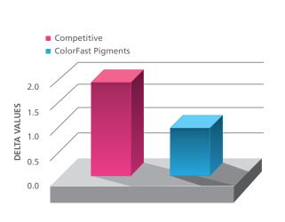
More than 45.0% difference in fade resistance after 5,000 hours of QUV exposure
