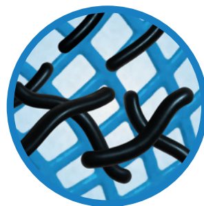
Traditional silicone products with free-silicone-fluid molecules
