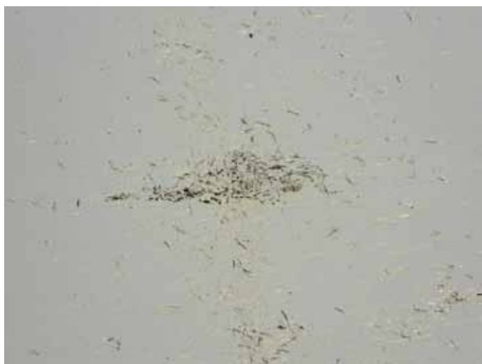
Figure A-1. Balling of fibers
