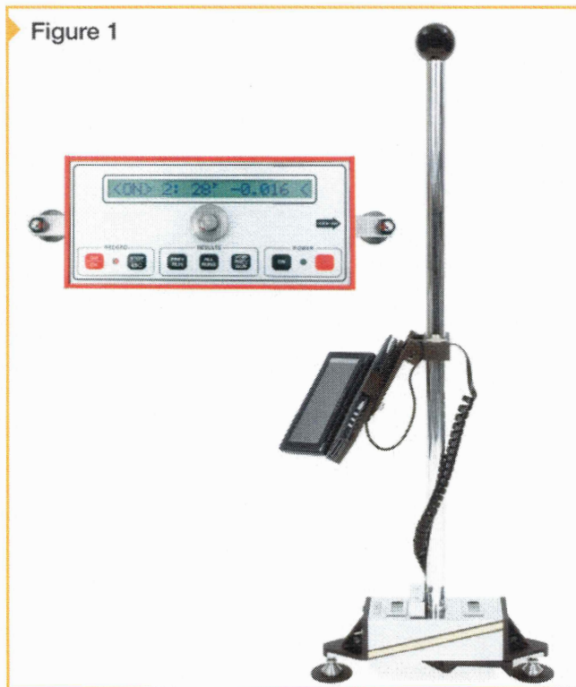
Figure 1 Apparatuses for measuring joint stability. These devices test the differential deflection of adjacent slab panels.
