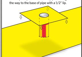
6. Tape the square piece to the pipe boot and around all edges.
