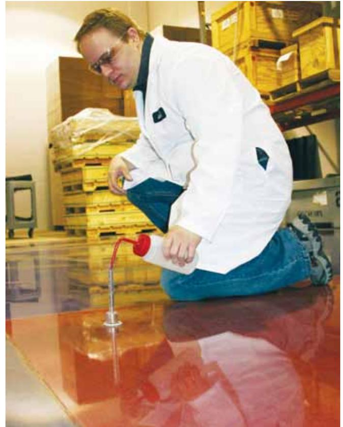
**Fig. 3 - Rilem Tube Test:** Consolideck® professionals are trained in the use of standardized performance tests. Here, a technician uses the kit's Rilem Tube to check the water-resistance of a Consolideck® Decorative Performance Floor.
