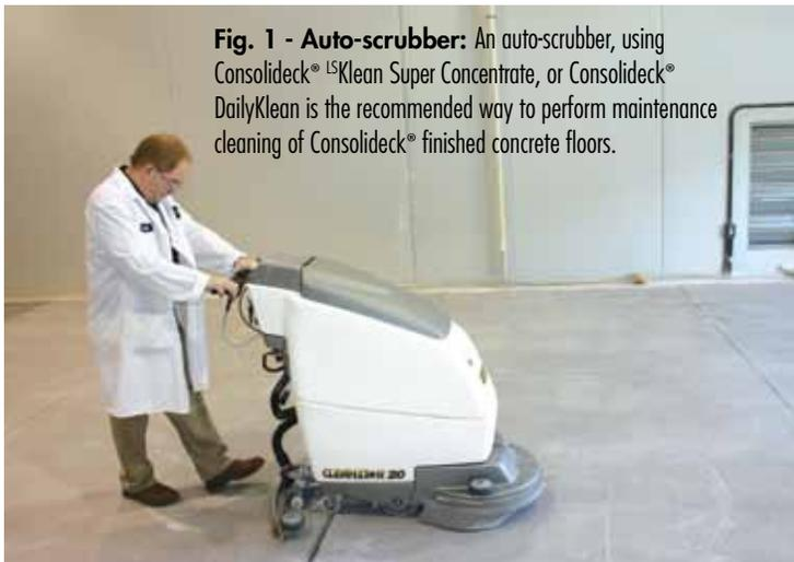
**Fig. 1 - Auto-scrubber:** An auto-scrubber, using Consolideck® <sup>LS</sup>Klean Super Concentrate, or Consolideck® DailyKlean is the recommended way to perform maintenance cleaning of Consolideck® finished concrete floors.
