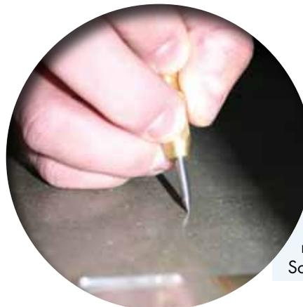
**Fig. 4 - Hardness test:** Here, a hardness pick is used to test the hardness of a honed performance floor, as measured on the Mohs Scale.
