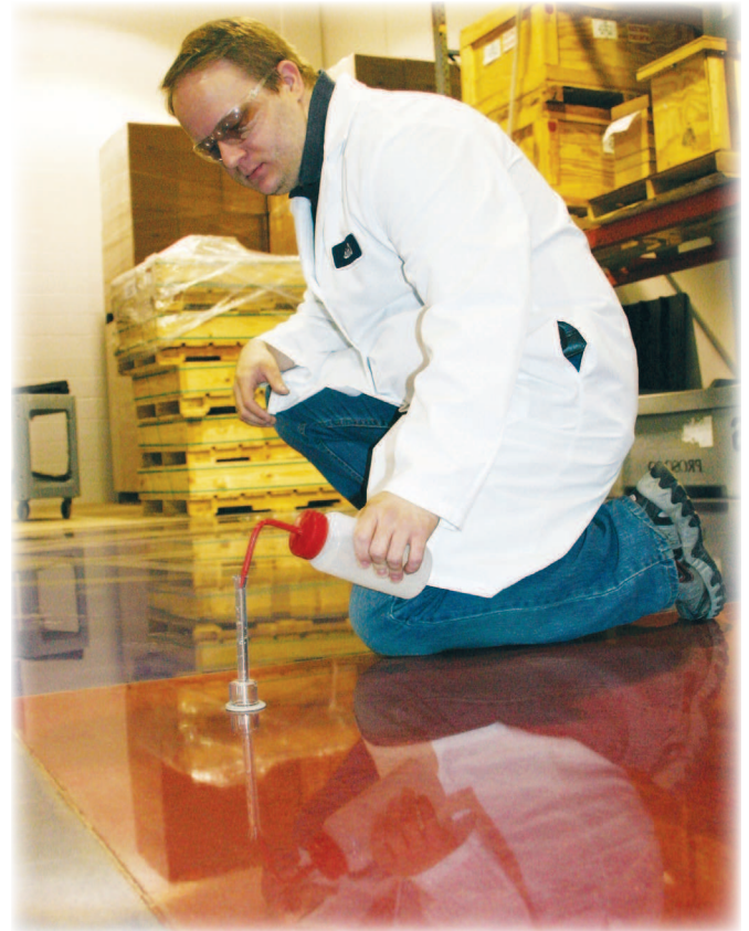
Fig. 3 - Rilem Tube Test: Consolideck® professionals are trained in the use of the standardized performance test kit. Here, a technician uses the kit's Rilem Tube to check the water-resistance of a Consolideck® Decorative Performance Floor.
