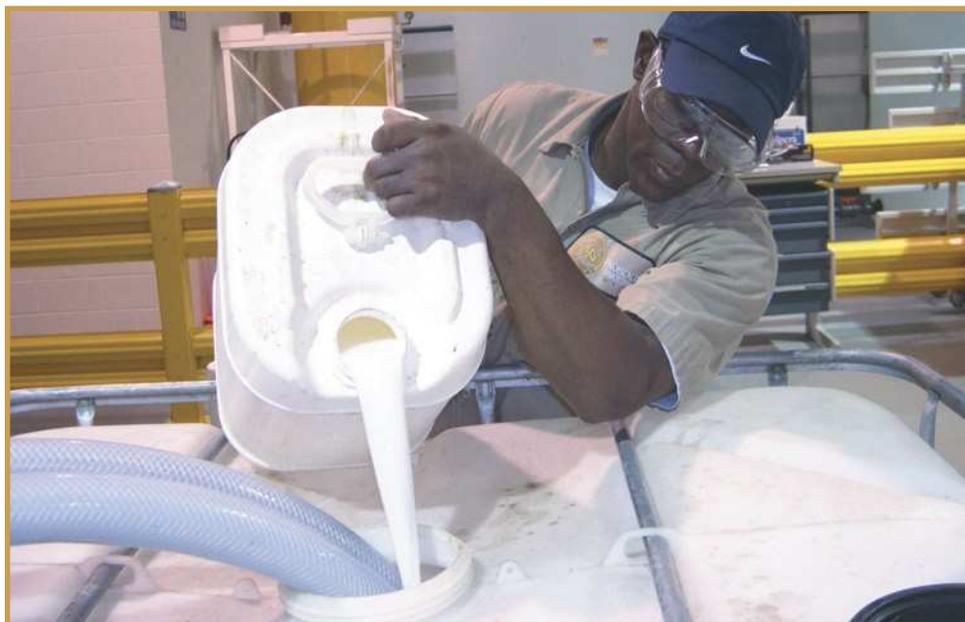
*Production Technician Willie Dickson pours the milky rinse water drained from a holding tank into a fill tank, where, instead of going down the drain, it will be used to make Sure Klean® Weather Seal Siloxane PD, a water repellent for masonry and concrete*
