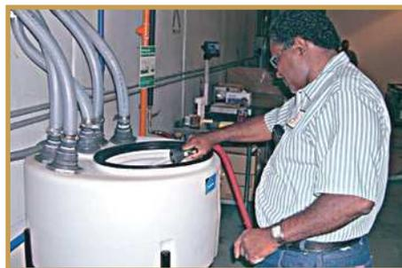
*Plant Manager Houston Williams rinses out a holding tank between making batches of Sure Klean® Weather Seal Siloxane PD, a water repellent for masonry and concrete. After rinsing the tank, the water will be drained and used again in making more Siloxane PD.*
