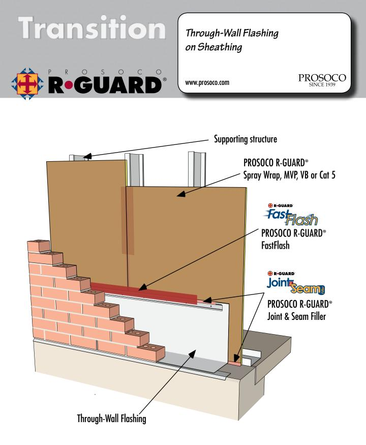
Through-Wall Flashing on a Spandrel Construction
