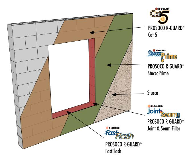
Rough Opening with Wood Buck Installation using Joint & Seam Filler, FastFlash, and Cat 5
