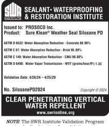
NOTE: The SWR Institute Validation Program uses standardized testing for validation purposes, including testing on CMU. PROSOCO <u>does not</u> recommend the use of Siloxane PD on CMU. Please reference the Substrate Chart on page 2.
