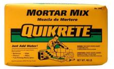
until a firm, workable consistency is achieved. The ideal mortar consistency has been achieved when a  $\frac{1}{2}$  in (13 mm) thickness of mortar will not fall off your trowel when held in a near vertical position. If more water is needed, add small amounts at a time and continue to mix until the desired consistency is achieved. The maximum water content is expected to be below 6 quarts (5.7 L) for each 80 lb (36.2 kg) bag and 4-1/2 quarts (4.3 L) for each 60 lb (27.2 kg) bag)
