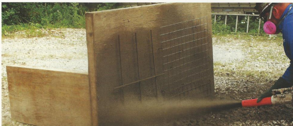
Fig. 5: Preparation of a shotcrete test panel
