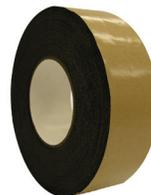
Butyl Seal is a double-sided reinforced aggressive black butyl rubber tape used to join panels of polyethylene and polypropylene together by overlapping the edges and applying Butyl Seal in between. It is also used to adhere to concrete walls and footings when properly prepared. Butyl Seal is non-hardening and flexible.
