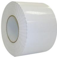
VaporBond™ Tape is a white single-sided tape that combines a heavy-duty, weather-resistant polyethylene backing with an aggressive rubber adhesive. VaporBond™ Tape offers excellent seaming capabilities for our materials with an "Easy Tear" feature to reduce installation time. TVB4 has a WVTR of 0.18 perms per ASTM D3833. Typical applications include vapor retarders, covers and liners.
