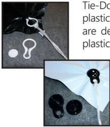
Tie-Down Buttons and Tarp Grabbers help keep plastic sheeting securely in place. Tie-Down Buttons are designed to eliminate traditional grommets in plastic sheeting up to 10 mil thick and are reusable plastic fittings that are easy to install in any position. Tarp Grabbers are up to 4 times stronger than a brass grommet and are typically used in heavier plastic sheeting from 10 mil to 30 mil thick. Great for equipment covers, large storage covers and truck tarps.
