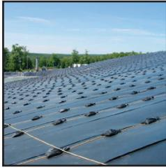
Dura♦Skrim® reinforced sandbags are used to secure large covers and liners to prevent wind damage. Sandbags are produced with strong Dura♦Skrim® 8 & 12 mil reinforced polyethylene. These 15" wide x 24" long bags are designed to hold 35 lbs. Sandbags are also available in other VIAFLEX reinforced materials with minimum order requirements. 11.8" Cable Ties are also available.
