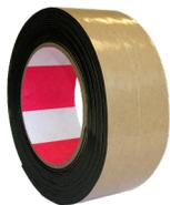
VaporBoot™ Tape is a single-sided elastomeric butyl tape used to complete pipe boot installations (sealing the boot to the pipe). The 100% stretchable butyl adhesive features excellent adhesion values and 3-D stretching that can be easily molded to multiple surfaces without any creases and folds.
