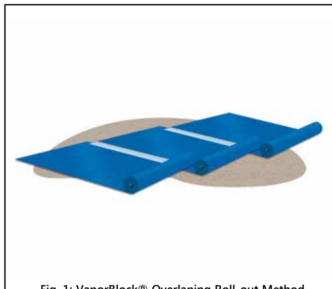
Fig. 1: VaporBlock® Overlapping Roll-out Method
