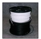
Raven Welding Rod is used for field seaming, repairs and detail work, such as installing pipe boots. Packaged in 25 lb spools, it is available in 4mm and 5mm sizes to fit most brands of extrusion guns. Raven Welding Rod is made from a thermally UV stabilized LLDPE resin and is available in both black and white to correspond with the color of geomembranes being utilized.
