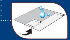
After watering the surface again, roll out the next layer of Transguard<sup>®</sup> 4000, making sure there is at least 4"- 6" overlap.
