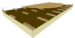
Multi-Layer Insulation Systems - Rmax recommends two layers of insulation whenever the total insulation requirement exceeds 3.0" to reduce thermal bridging, moisture migration and system movement. Multi-Layer systems utilize Multi-Max° FA-3 or Ultra-Max° as the bottom layer prior to installing the Multi-Vent Nailable Base-3. Joints should be offset between the insulation layers as well as between the insulation and cover board.
